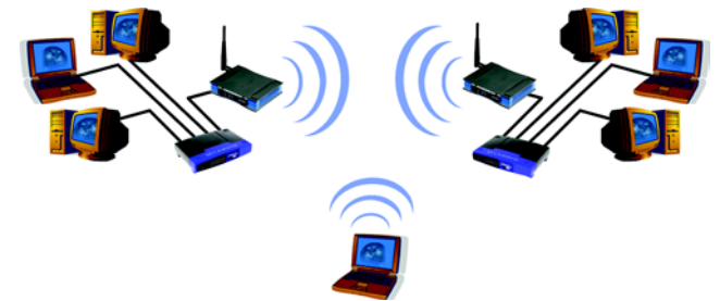
Figure 2-3: Network Using Wireless Bridging
